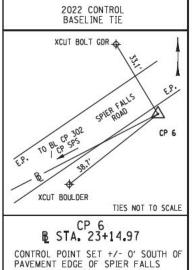
CONTROL POINT SET +/- O' SOUTH OF PAVEMENT EDGE OF SPIER FALLS ROAD AND +/- 650' EAST FROM THE SPIER FALLS ROAD CULVERT
